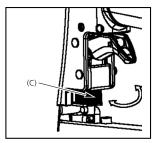
3. To sink a nail deeper, turn the wheel (C) to left to the extent desired
