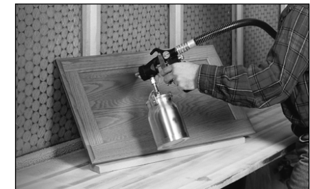
Spraying cabinet doors
