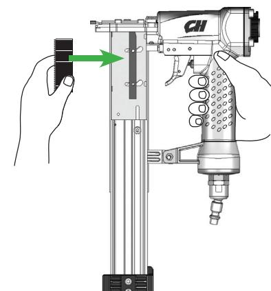
**Load** pins with points all the way into the groove.
