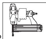
7. Pull the trigger and depress the work contact element (WCE) against the work surface. The tool **MUST NOT OPERATE**.
