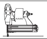
6. Remove the tool from the work surface. The Work Contact Element (WCE) must return to its original down position. The tool **MUST NOT OPERATE**. Do not use the tool if it operates while lifted from the work surface. Personal injury may result.
