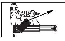
3. Make sure the trigger and work contact element (WCE) move freely up and down without sticking or binding.
