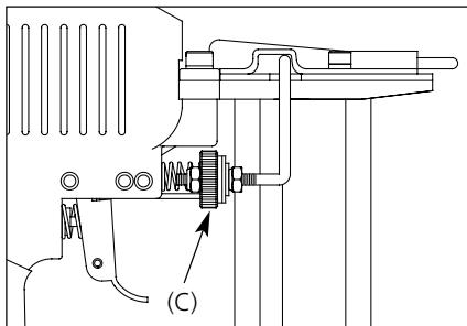
3. For deeper penetration, turn the wheel (C) to left to the extent desired.
