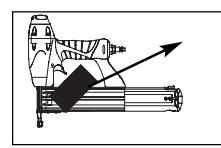
**WARNING** *Failure to remove all fasteners will cause the fasteners to eject from the front of the tool.*
