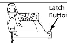
2. Push in on the latch button. Pull back on the magazine cover.
