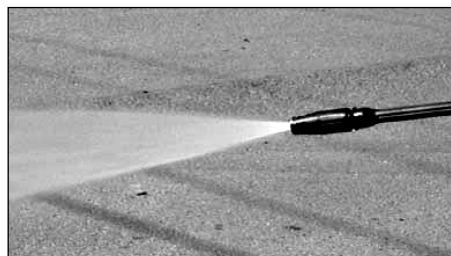
Figure 14 - Wide fan pattern
