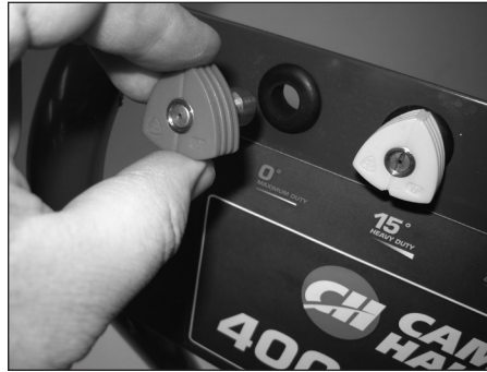
Figure 3 - Insert spray tips into the holder
