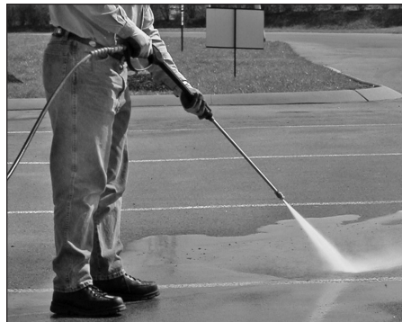
Figure 14 - Optimum angle to cleaning surface
