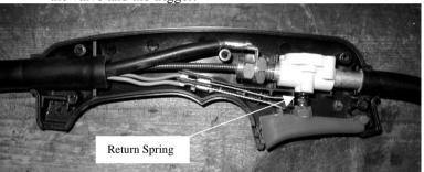
22. Replace the other torch half and reinstall the five screws.
