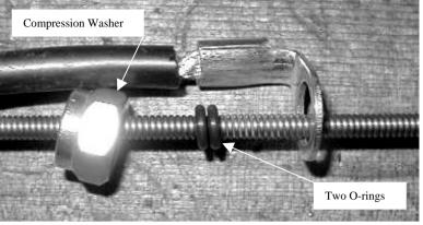
14. Insert wire liner into swan neck, making sure welding cable ring connector is in place over swan neck.
