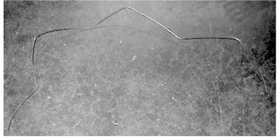
9. Insert one foot of bent welding wire into wire liner at drive deck.
