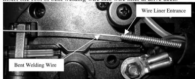
10. Place new wire liner over other end of welding wire.
