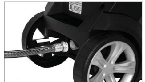
Figure 13 - Attach garden hose to unit (model PW1825)
