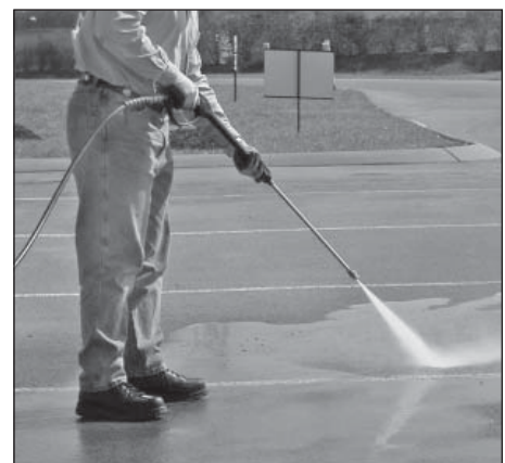
Figure 22 - Optimum angle to cleaning surface
