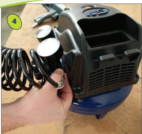
Attach air hose to air compressor.
