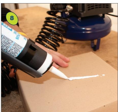
Test a caulk bead by pulling trigger and running a bead on a piece of cardboard. Adjust the air pressure, size of tube end and speed as needed. Do not exceed 20 psi.
