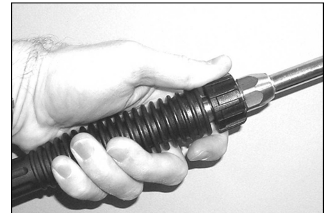
Figure 6 - Attach lance to gun
