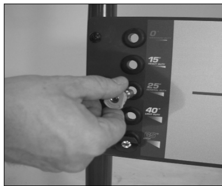
Figure 3 - Insert spray tips into the holder
