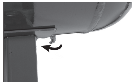
Figure 10 - Manual Tank Drain
