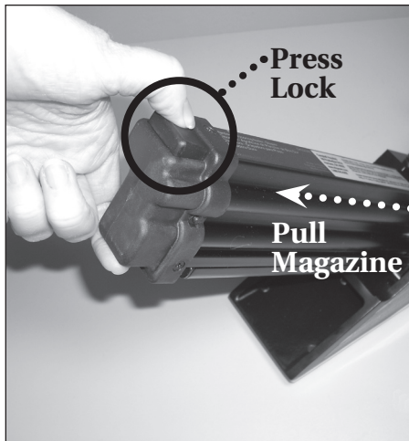
Figure 16 - Press the lock and pull the magazine door
