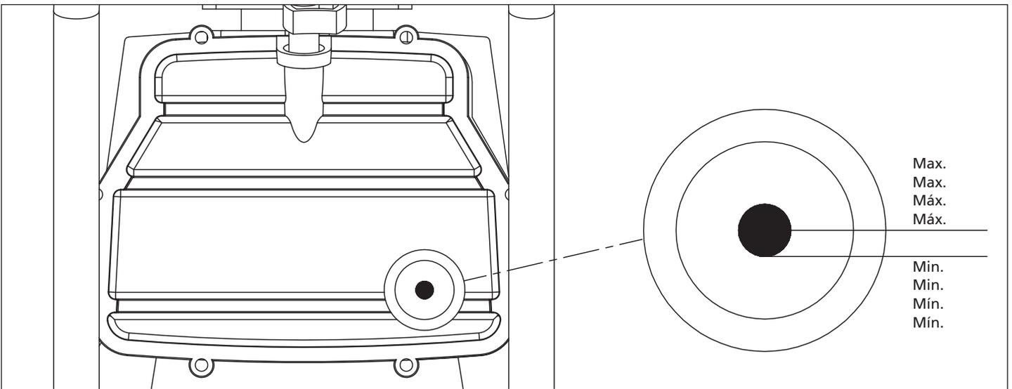
**Figure 4 - Proper oil level**
