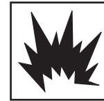
Risk of Explosion
